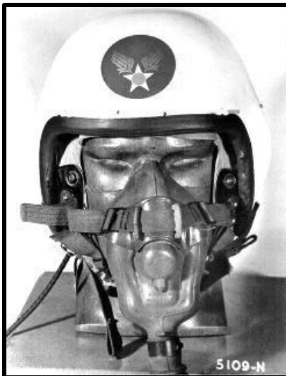
Figure 38: A front view of the prototype P-2 helmet with MS22001 mask.
