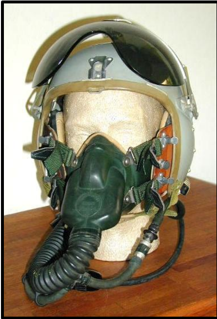
Figure 23: An extremely rare helmet and mask, the Russian ZSh-2 and KM-24, copies of the USAF P-3 and MS22001 mask, 1955.
