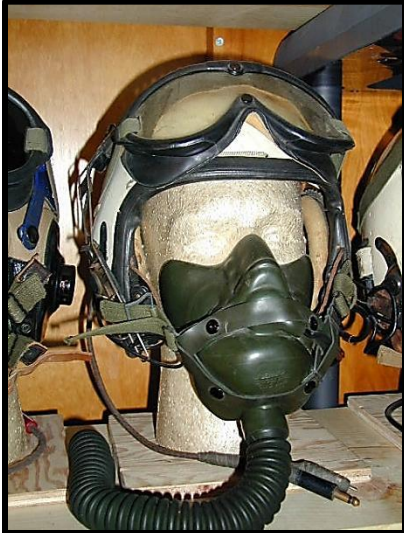
Figure 27: The USAF P-1 helmet, shown in use with an A-14 demand oxygen mask.
