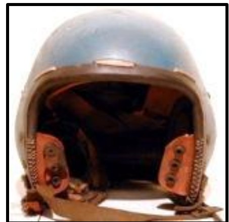
Figure 30: A front view of an upgraded (to P-1A status) P-1 helmet; note the characteristic cross-stitching on the edgeroll, signifying modification.
