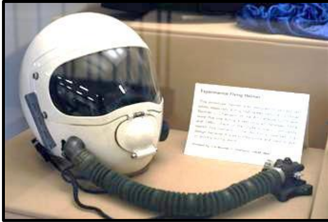
Figure 14: A rare HGU-20/P precursor design, experimental wind-blast helmet (USAF) 1960, on display at the National Air & Space Museum.
