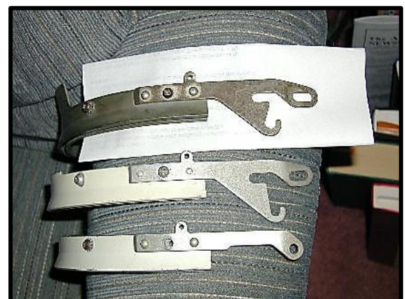
Figure 49: Top, 2nd gen short J-hook' from P-3; middle, longer 'J-hook' from P-4; bottom, P-4A & P-4B assembly.
