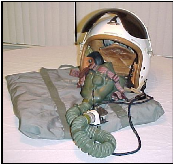
Figure 47: A nice P-4B helmet; note issue carry bag; the com cord is connected to the mask hose, but in this example, the cord keepers have failed.
