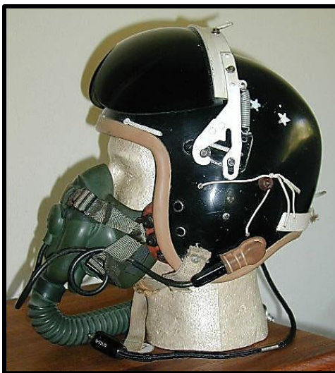
Figure 41: A P-4 helmet viewed from the left: note the higher visor position over eyes, due to the longer 'J-hook'.
