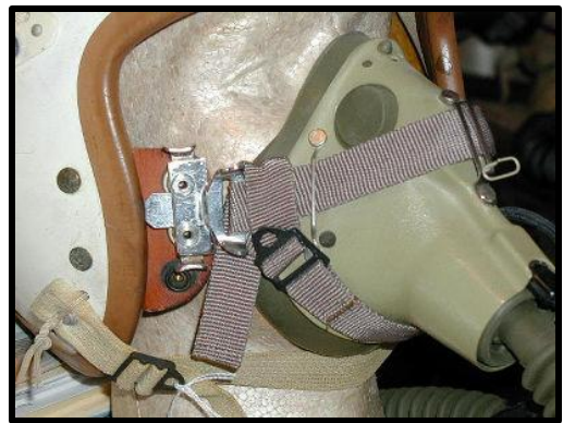
Figure 52: Rarely seen, a short bayonet receiver system that snapped onto P-helmet leather mask tabs.
