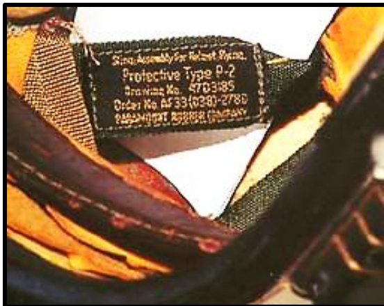
Figure 55: The erstwhile 'false P-2 helmet' sling that was used as a replacement in P-1A and P-1B helmets.
