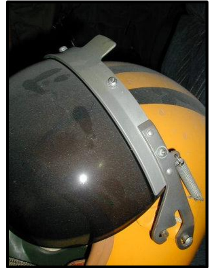
Figure 47: Note short side latching 'J-hook' on an early P-3 (2 nd gen visor yoke).
