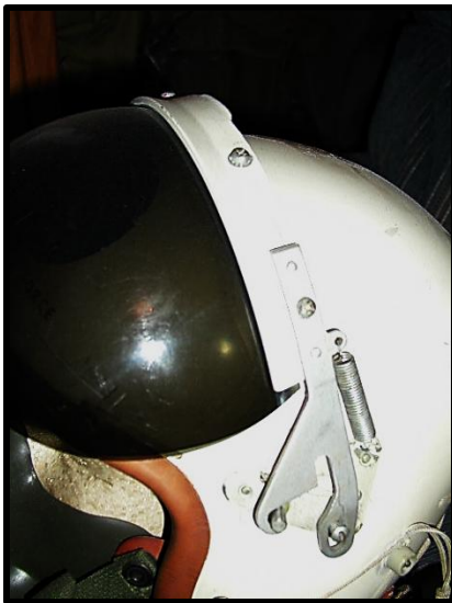
Figure 48: Note longer 'J-hook' on a P-4 (3 rd gen visor yoke)
