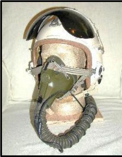
Figure 10: The USAF P-4B, 1959, last of the P-series helmets.
