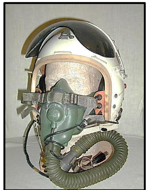
Figure 46: Your first visual clue to P-4A identity is the pigtail com-cord coming from rear of helmet shell (the P-4B did away with this feature).
