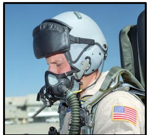
Figure 25: Another rare helmet, the two-part modular helmet design, flight tested at DFRC (used to investigate multi-mission modes).
