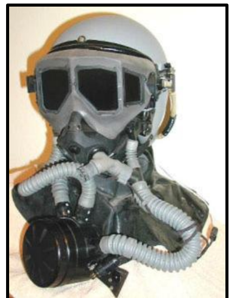
Figure 15: USAF TLSS (Tactical Life Support System) helmet, NBC configuration (late 80s).
