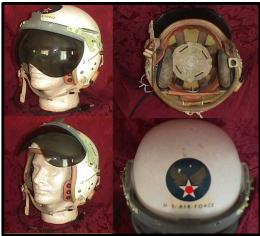
Figure 44: Another composite 4-view of a P-4 helmet.
