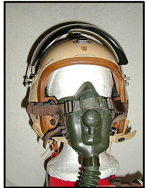
Figure 46: The P-4B used a com cord that connected to aircraft via the oxygen mask .
