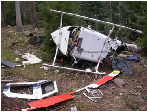
Aircraft impacted on left side after 100' fall... No serious head injuries to the survivors.
