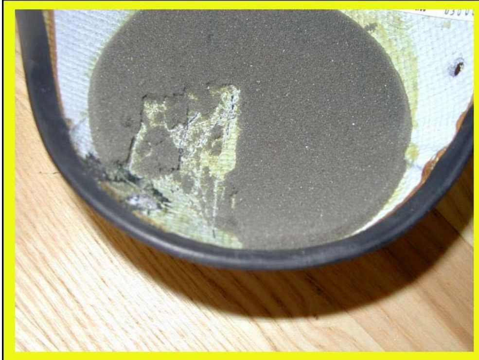
Ear cup chaffing pads should be intact and pliable. If they deteriorate – replace as soon as possible.
