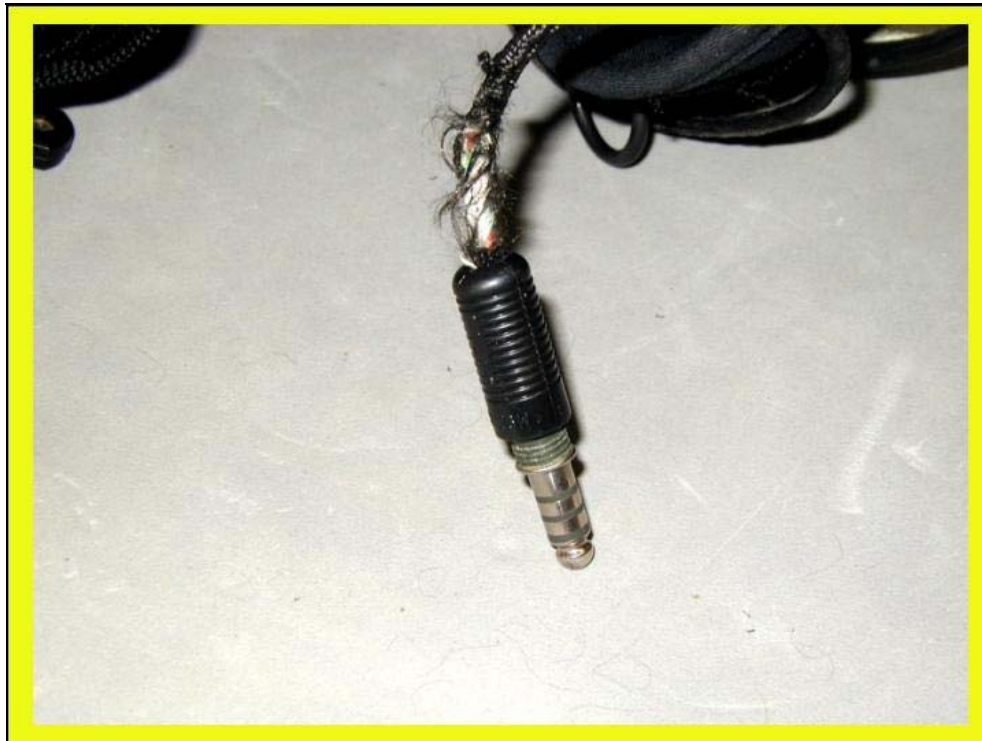
Frayed casings for microphone cords can allow the cord to become damaged. Replace as soon as possible.
