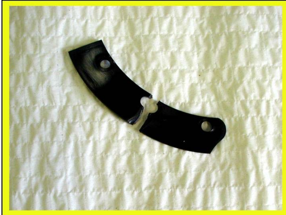
Broken visor tracks will make it difficult to operate your visor. Replace as soon as possible.
