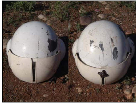
Aircraft impacted on left side after 100' fall... No serious head injuries to the survivors.
