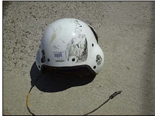
Two rotor blade strikes to the helmet... No permanent head injuries.
