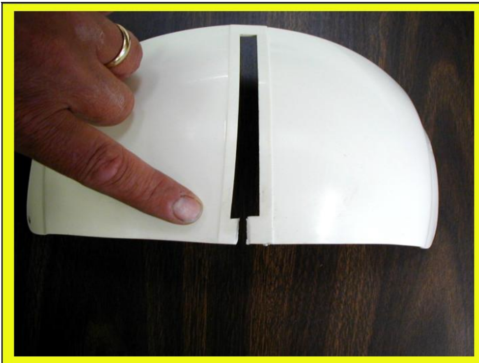
Cracked or broken visor housings make it difficult to operate your visor. Replace as soon as possible.
