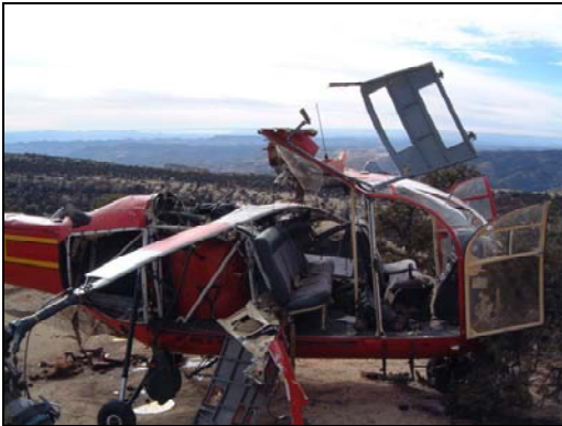
Main rotor blade struck 4 passenger's helmets... Only one serious injury.
