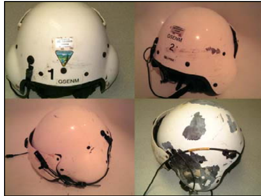
Main rotor blade struck 4 passenger's helmets... Only one serious injury.
