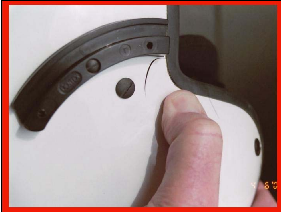
Helmet cracks often occur around the ear cup. A crack or other serious damage to a helmet's shell makes the helmet unserviceable.
