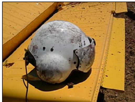
After impact the airplane rotated 180°... No head injuries.
