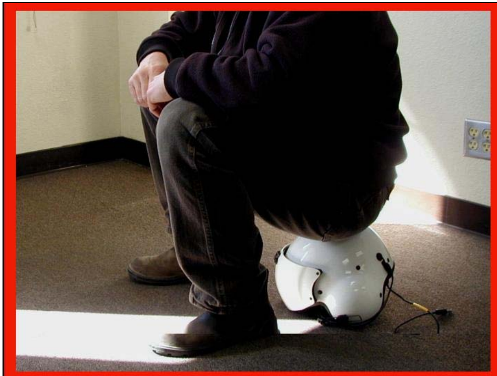
Most cracks in the helmet's shell are found on the ear cups, don't sit on your flight helmet.
